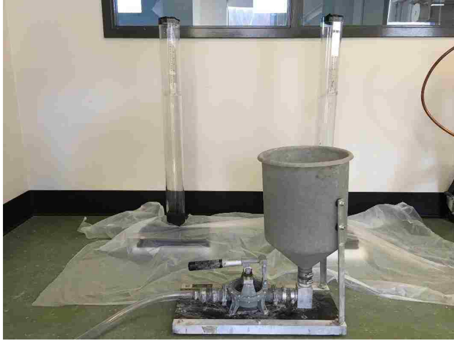
Figure 4.1 - Photograph of grout pump used to pour grout into test tube.
