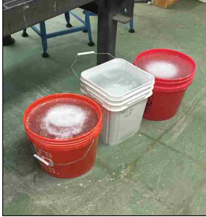
Figure 5.1 - Specimens CG (left), B10 (middle), and B20 (right) during curing.
